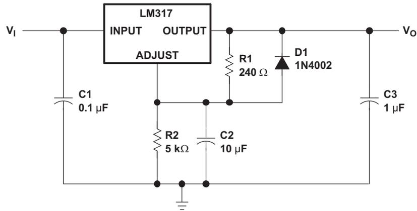
**Figure 13. Adjustable Regulator Circuit with Improved Ripple Rejection**
